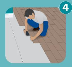
Lay the vinyl floor in the same direction as the underlayment or at a 90 degree angle, follow LVT flooring manufacturer's recommendation. Picture shows vinyl floor and underlayment laid in same direction
