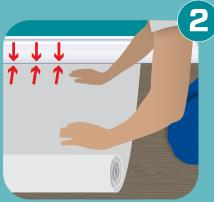
Lay the first length of underlayment tightly against the wall across the full width of the room
