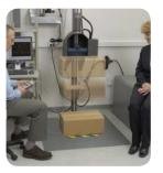
Verification and Validation - We will then test the sample package using a variety of atmospheric and standardized methods, including ISTA, ASTM, ISO and NMFTA.
