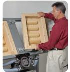
Tooling - When you are ready to implement your new Instapak® molded solution, Sealed Air will manufacture custom-made production tooling ready for installation.
