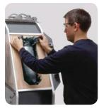
When placed into the mold enclosure, the bag is drawn in by an on-board vacuum.
