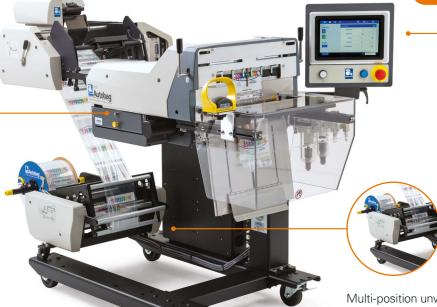
Multi-position unwind with tension control simplifies changeover
