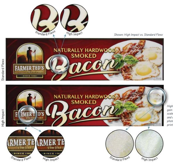
High Impact printing reduces dot gain improving the overall tonal scale and range for better contrast and detail. The result - a more photo-realistic, premium quality print versus standard flexo.
