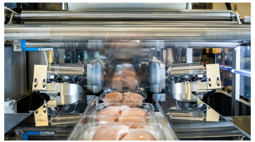
CRYOVAC® brand overwrap film with recycled content running in a fresh poultry application
