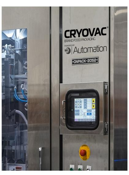
CRYOVAC® brand vertical form-fill-seal system
