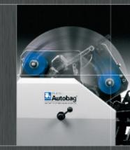
Festoon control, a PI 412cw exclusive, allows printer to run continuously—independent of the bagger—ensuring speed and print registration.
